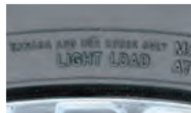
Figure 1—Light Load molded into sidewall
