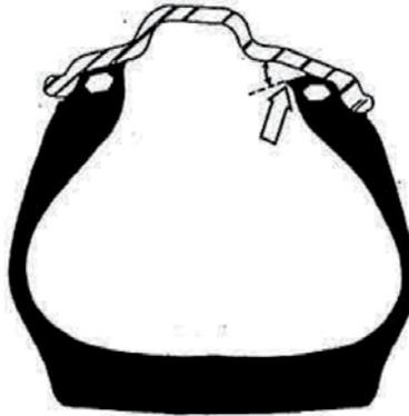
Extreme stress may be placed on beads forced into the rim flange in a distorted manner, which may cause fatigue in tire components and result in tire failure.
